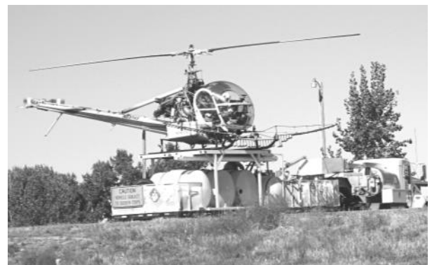
Vegetation Control — Sky Copters Inc. sprays new tree growth in low water areas of Spillway Bay at Lake McConaughy (top). At bottom, the helicopter lands on a trailer to refill its tank with herbicide.
